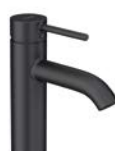
KLUDI BOZZ Single lever basin mixer 100 DN 15 with PUSH-OPEN waste G 1 1/4 and without pop-up waste* spout height lower edge = 100 mm
